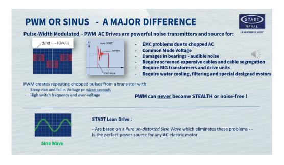
Here we are into the details of the IGBTs high frequency switching and so on. And the core of the challenges seen in those PWM drives.
