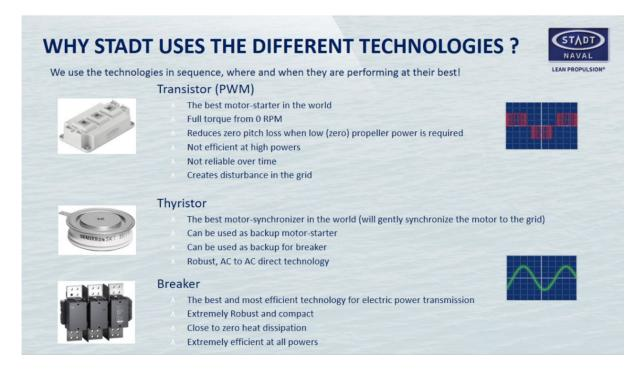
We are combining transistor technology with thyristors and breakers. In a symbiosis, you could say. To obtain the qualities we are aiming for.
