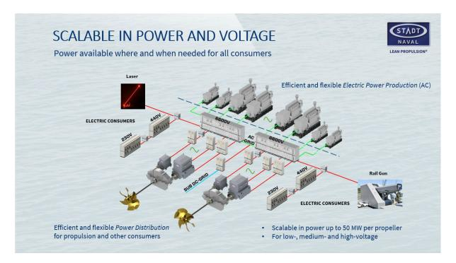
Here we see a combination of a high-power solution with 6600 V AC.
