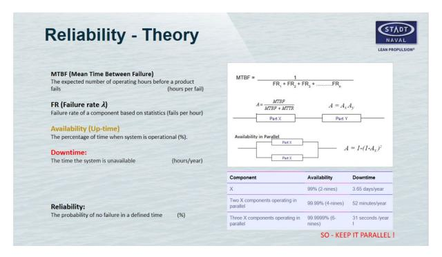
Here we are talking about reliability and why we have such high reliability. It's because instead of a long chain of serial-connected components, we go in parallel.
